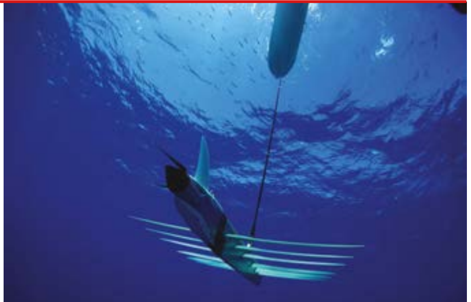
Liquid Robotics' Wave Glider can be configured with acoustic modems or towed hydrophones, meaning it can act as a gateway or communications hub for UUVs. (Photo: Liquid Robotics)
